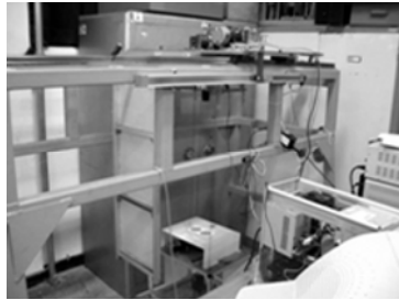
(a) Anti-sway system for container cranes
